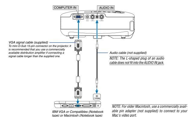
NOTE: The projector is not compatible with video decoded outputs of either the NEC ISS-6020 and ISS-6010 switchers.
